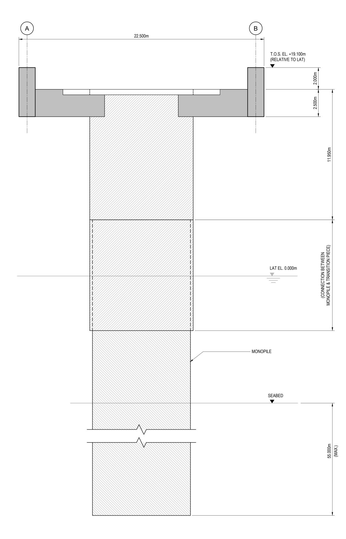
LEFT ELEVATION ( Scale 1:200 ) NOTE : EXPECTED WATER DEPTH AT OSP LOCATION RANGES FROM 13m TO 24m RELATIVE TO LAT
